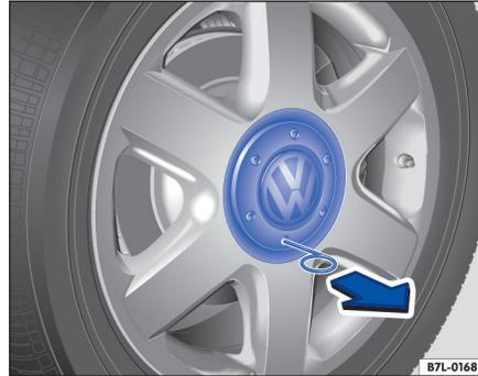
Fig. 181 Pulling the hubcap off.
