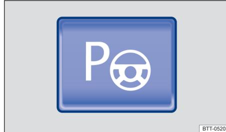
**Fig. 119** In the lower center console: Button for switching on the Park Assist system.
