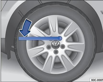
Fig. 185 Changing a wheel: Loosening the wheel bolts.
