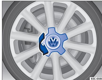
Fig. 182 Twisting the hubcap off.
