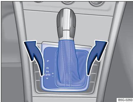
Fig. 104 Removing the selector gate cover.
