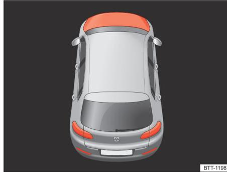
**Fig. 168** In the instrument cluster display: Engine hood open or not properly closed.
