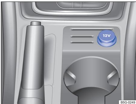
**Fig. 138** In the lower center console: 12 Volt socket (vehicles with parking brake lever).
