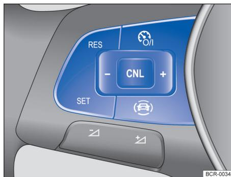
**Fig. 107** Left-hand side of the multi-function steering wheel: Buttons for operating the cruise control.
