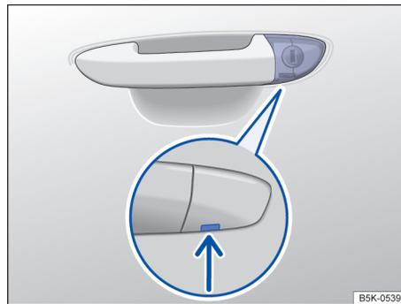
**Fig. 53** Driver door: Concealed lock cylinder.
