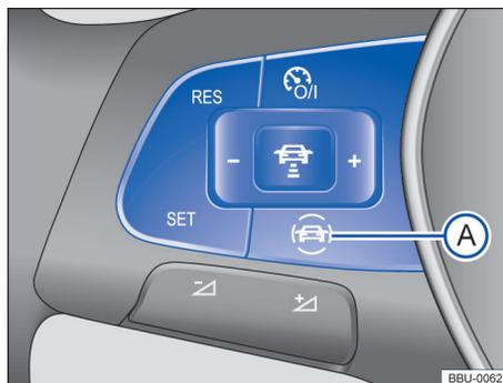
**Fig. 17** On the multi-function steering wheel: Driver assistance systems button.
