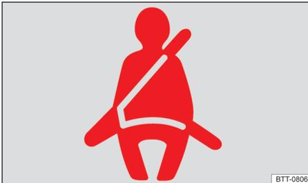
Fig. 22 Warning light in the instrument cluster.
