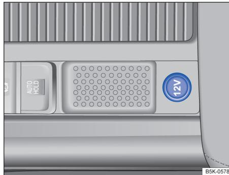
**Fig. 139** In the lower center console: 12 Volt socket (vehicles with electronic parking brake).
