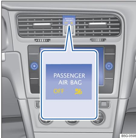
**Fig. 33** In the instrument panel: PASSENGER AIR BAG OFF
