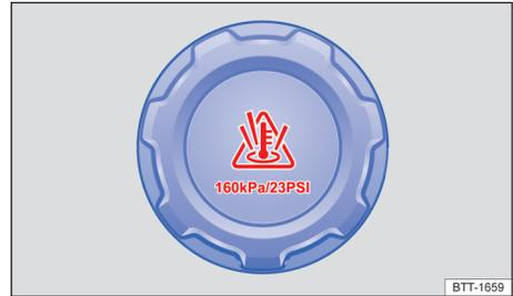
**Fig. 173** Coolant expansion tank cap in the engine compartment.
