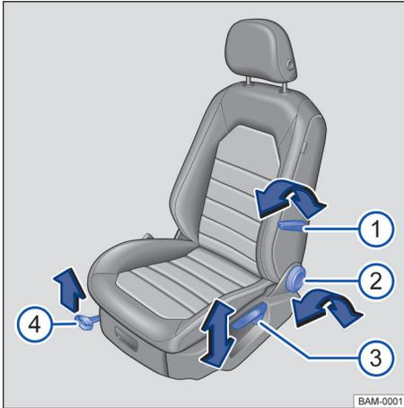
**Fig. 68** Driver seat: Manual seat adjustment controls.
