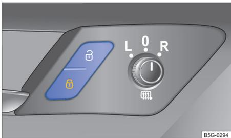
**Fig. 52** In the driver and front passenger doors: Power locking switch.
