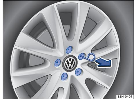
**Fig. 184** Pulling cover caps off wheel bolts.
